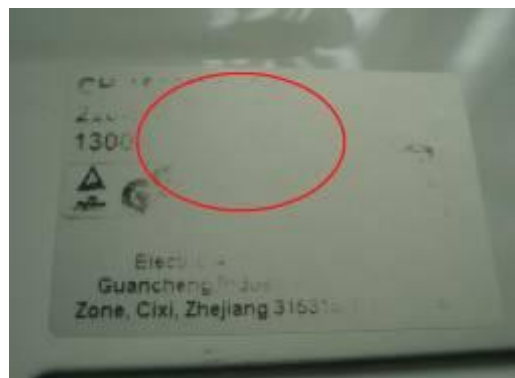
Photo-30 Use alcohol to do rubbing test on surface of rated label with force of 300g for 15 times, letter on the label was erased.
