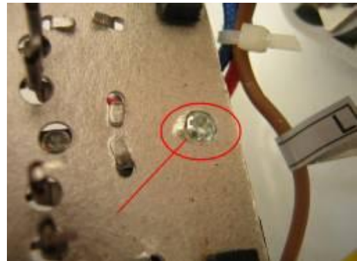
Photo-38 Screw gets into the mica plate, and cause the mica plate loose out.
