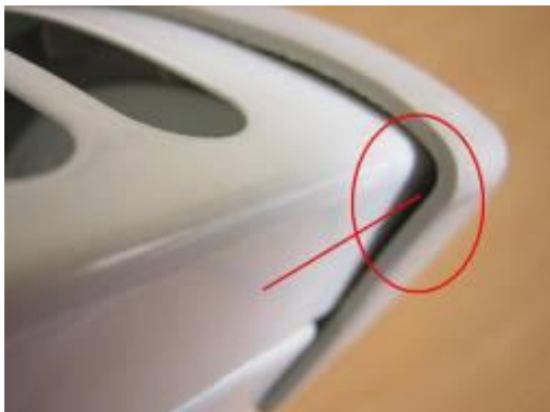
Photo-35 Handle of unit assembly construction check: Gap about 3.7- 4.0mm between handle and unit outer shell.-2
