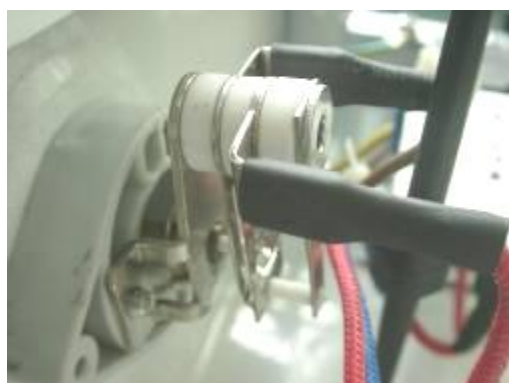
Photo-43 Connection terminal fixing on thermostat check.
