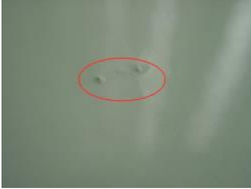
Photo-25 Coat on outer shell surface bulgy.
