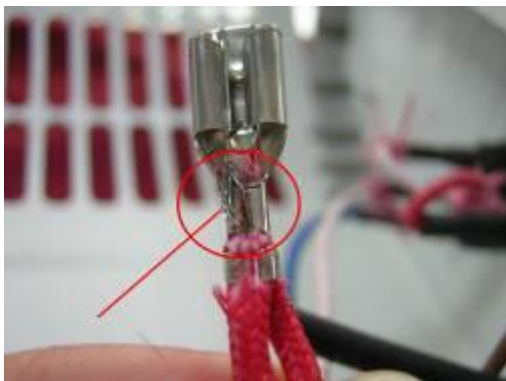
Photo-53 Found that connection wire can not fix in the terminal completely.
