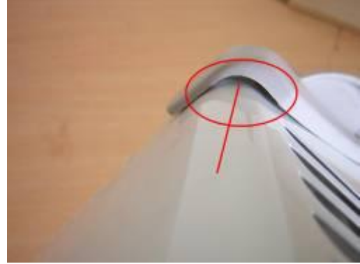
Photo-34 Handle of unit assembly construction check: Gap about 3.7- 4.0mm between handle and unit outer shell. -1
