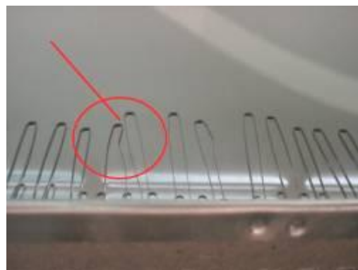
Photo-48 Heating element fixing status: Distance between heating elements not even, distance between some of the heating elements is only 0.2mm.
