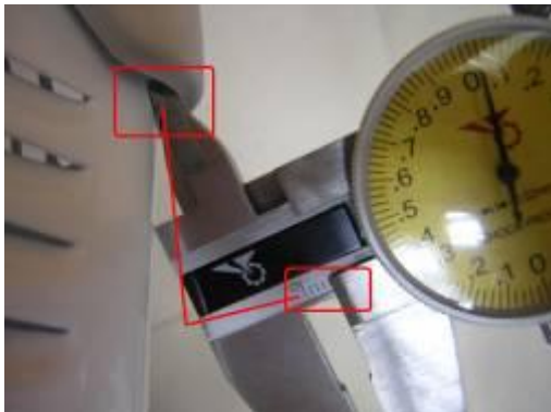
Photo-37 Handle of unit assembly construction check: Gap about 3.7- 4.0mm between handle and unit outer shell. -4
