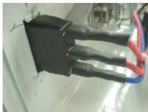
Photo-44 Connection terminal fixing on power switch check
