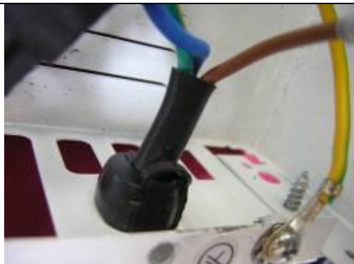
Photo-41 Power cord and cable gripper fixing status check.
