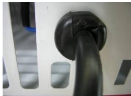
Photo-40 Power cord fixing on outer shell status check.
