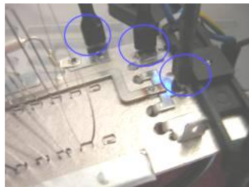
Photo-46 Connection terminal fixing on heating element check.
