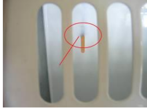
Photo-26 Poor painting of inner bracket buckle position.-1
