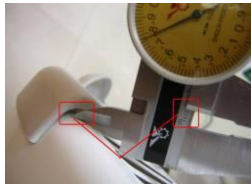
Photo-36 Handle of unit assembly construction check: Gap about 3.7- 4.0mm between handle and unit outer shell. -3
